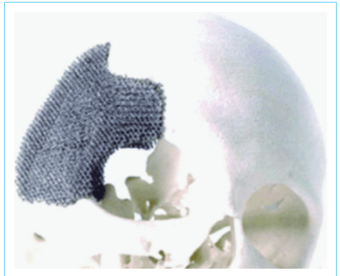
Figure 9 – Ti6Al4V skull flap obtained through a powder bed fusion process (credit Murr et al. [4])
