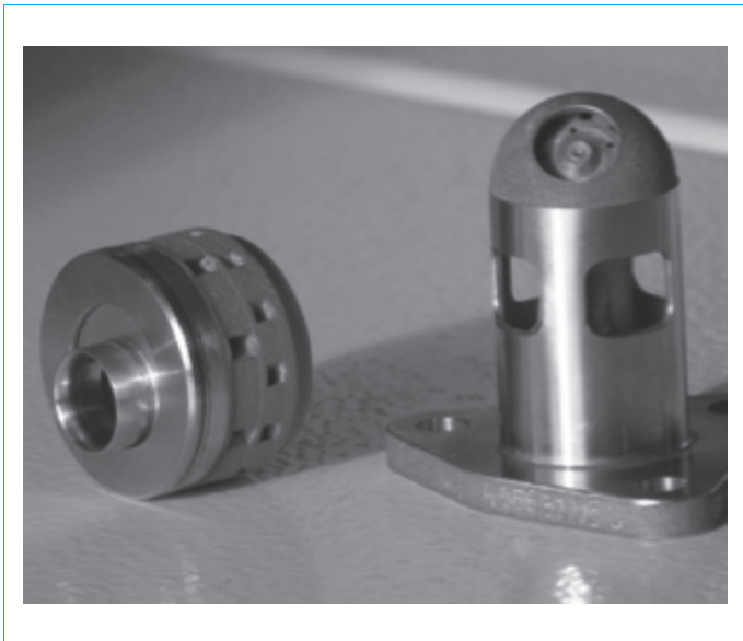
Figure 8 – Fuel injector and combustion chamber swirl generator (credit Turbomeca – R. Bertrand)
