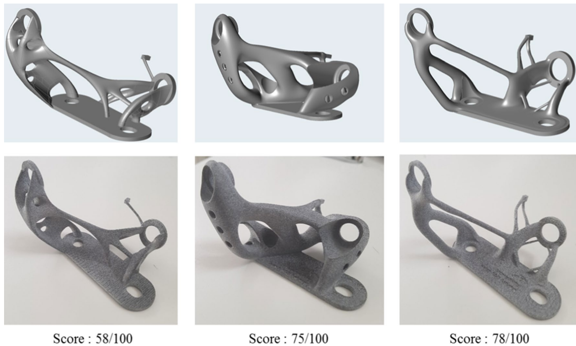
Fig. 8 Preview of different challenge solutions with their ranking score: CAD (up) and printed (bottom) versions
